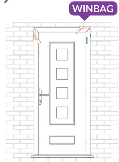
Insert and inflate the Winbag over the hinge side to compress the frame down onto the 5mm packer.
