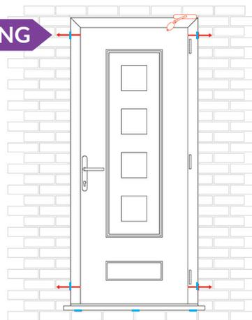
Drill and fix through the top of the closing side, through a packer.
