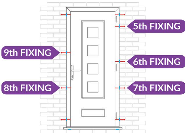
Drill and fix through a packer for the remaining 5 fixing positions. After each fixing check the mech to ensure that nothing has moved and the door still functions correctly.
