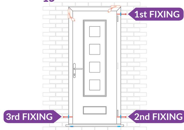
Make a fixing as close as possible above the top hinge through the packer. Drill and fix below the bottom hinge through the packer. Drill and fix through the bottom of the closing side, through the packer.
