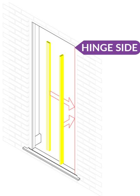
Plumb the hinge side. Leave a small gap to the plaster line to allow for setting the viewing gap.
