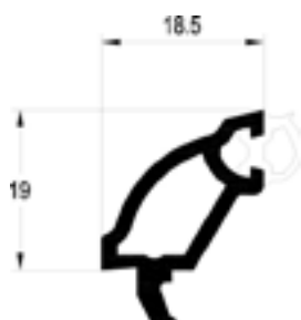
Co-extruded Glazing Bead 18.5 For 28mm sealed units Art.546572
