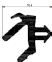
Universal Repair Gasket for IG Profiles Art.506140
