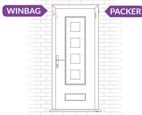
Pack between the brickwork and frame just above the top hinge and insert and inflate the Winbag on the opening side of the frame and inflate enough to hold the packer in place.
