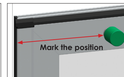
Mark the position with pencil
