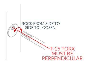
1. Use a T-15 TORX and insert into the TOP keep. Rotate to slightly move the adjustable keep towards the Grey brush pile. Check the Mech, then repeat if necessary.
