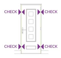
4. Check the lock side gaps are equal to the hinge side gaps.
