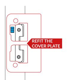
**9.**Refit and tighten x2 cross head screws.
