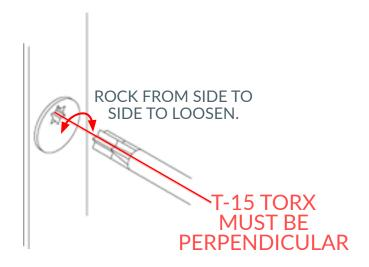
1. Use a T-15 Torx and insert into the TOP keep. Rotate to slightly move the adjustable keep towards the black Q-lon gasket.
