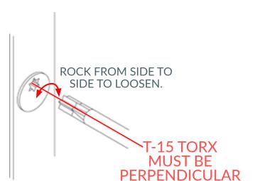
1. Use a T-15 Torx and insert into the top keep. Rotate to slightly move the adjustable keep towards the Grey brush pile. Check the Mech, then repeat if necessary.
