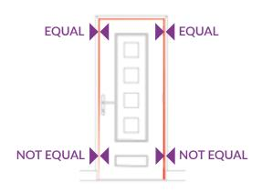
**3.** Check the side gaps at the bottom of the door.
