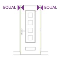
2. Check the side gaps at the top of the door. If the gaps are not equal repeat step 1 until they are equal.
