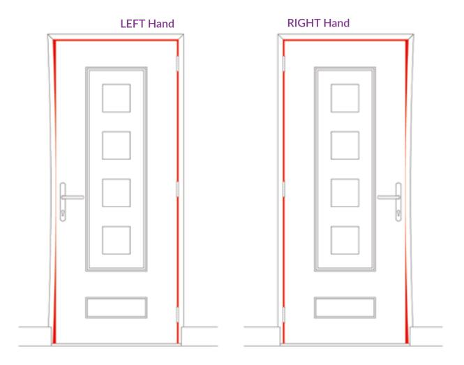
If the side gap changes more than 2mm along one side then the **frame** needs adjusting as this is a fitting issue.
