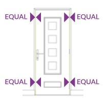
3. If the gaps are equal adjust the centre hinge exactly the same amount. If the Head gap is Parallel and within specification move on to check the viewing gap.
