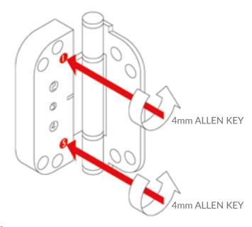
1. Top hinge use a 4mm allen key and turn 1 and 5 half a turn in an anti clockwise direction.
