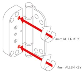
1. Use a 4mm allen key and turn 1 and 5 half a turn in a clockwise direction.
