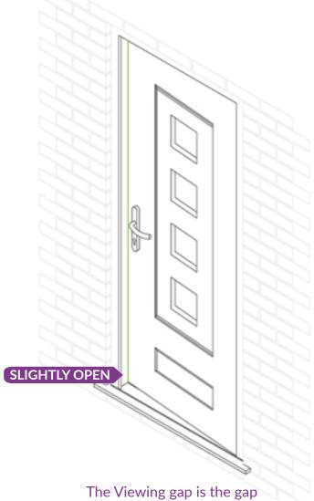
The Viewing gap is the gap between the sash and the frame when the door is slightly open as shown.
