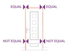
**3.** Check the side gaps at the Bottom of the door.
