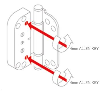
1. Adjust the top hinge use a 4mm allen key and turn 1 and 5 half a turn in a anti clockwise
