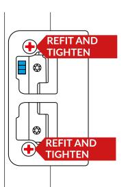
10. Refit the centre keep to the door frame and check the operation. Adjustments can be made as in previous
