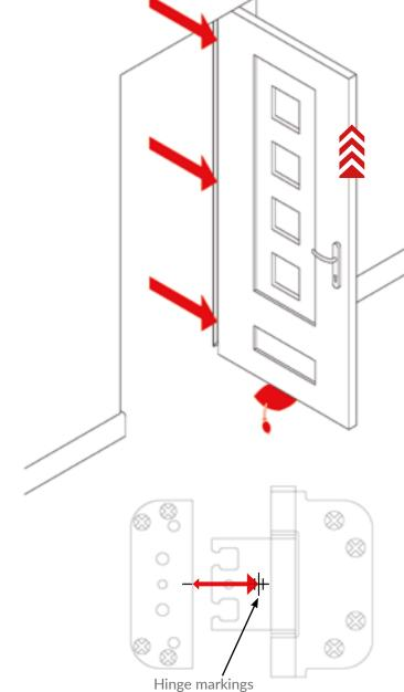
When lifting the sash, it's easier if you tighten the middle hinge first, to hold the sash and then do the top and bottom hinges as it works like a pivot so you can set the compression. Hinge markings are at approx. 2mm increments, to use as a guide.
