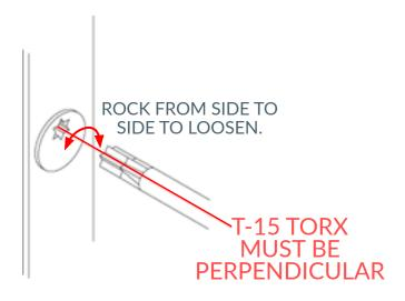
1. Use a T-15 TORX and insert into the TOP keep. Rotate to slightly move the adjustable keep towards the Black Q-Lon Gasket. Check the Mech, then repeat if necessary.
