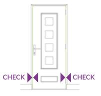
2. Check the side gaps at the bottom of the door. If the gaps are not equal repeat step 1 until they are equal.
