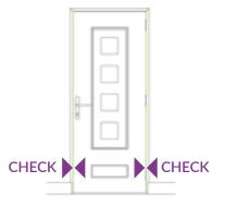
2. Check the side gaps at the bottom of the door. If the gaps are not equal repeat step 1 until they are equal.
