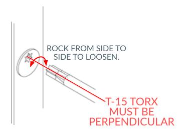
1. Use a T-15 Torx and insert into the top keep. Rotate to slightly move the adjustable keep away from the Black Q-lon gasket.
