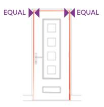
2. Check the side gaps at the top of the door. If the gaps are not equal repeat step 1 until they are equal.
