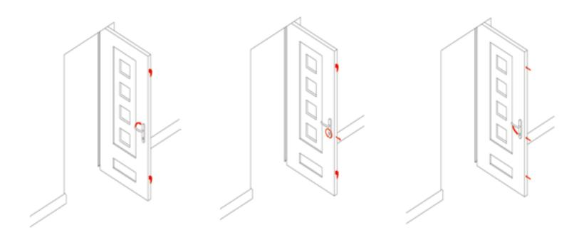
Open the door and then throw the hooks. Turn the key to lock, then unlock and retract the hooks.
