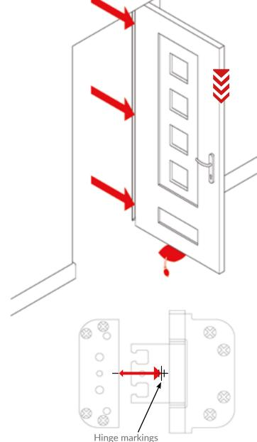
When lowering the sash, it's easier if you tighten the middle hinge first, to hold the sash and then do the top and bottom hinges as it works like a pivot so you can set the compression. Hinge markings are at approx. 2mm increments, to use as a guide.
