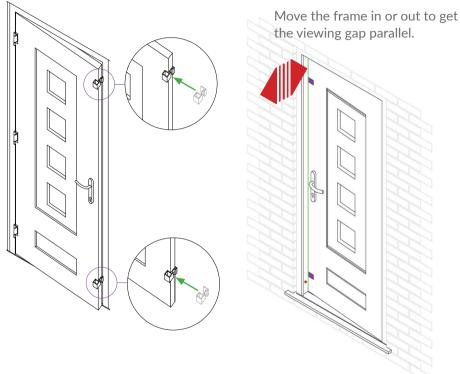
Place on the viewing clips to the top and the bottom of the sash. Close the door up to the frame and move the top part of the frame using the bottom fixing as a pivot, until both viewing clips are touching the frame- the viewing gap should now be parallel. When the viewing gap is parallel, clamp the frame with a winbag.
