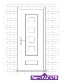
On the **hinge side** place a 5mm packer between the cill and the brick work. Offer the door into the aperture.
