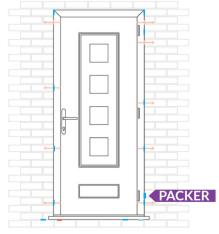
Packing directly behind the bottom hinge stops the weight of the door deflecting the frame in the future.
