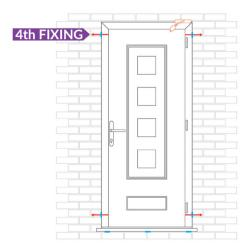
Drill and fix through the top of the closing side, through a packer.
