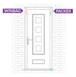
Pack between the brickwork and frame just above the top hinge and insert and inflate the Winbag on the opening side of the frame and inflate enough to hold the packer in place.
