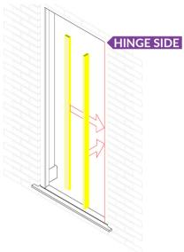
Plumb the hinge side. Leave a small gap to the plaster line to allow for setting the peep gap.
