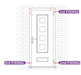
Make a fixing as close as possible above the top hinge through the packer. Drill and fix below the bottom hinge through the packer. Drill and fix through the bottom of the closing side, through the packer.
